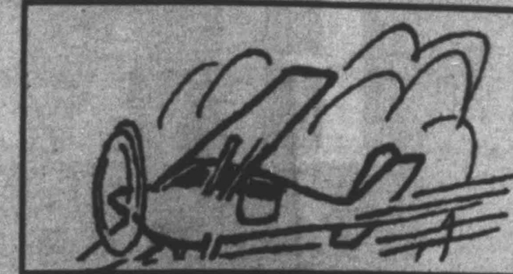
Most light planes are capable of taking off or landing in 90-degree crosswinds that are less than 20 percent of the airplane's power-off stall speed.
